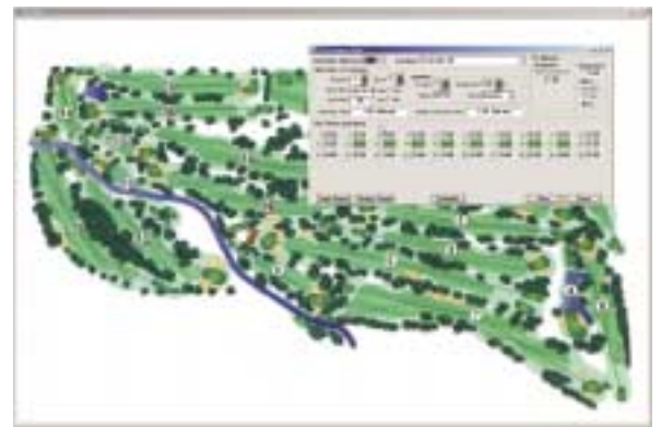
The custom map view provides instant access to all common control and programming functions for each hole of golf
